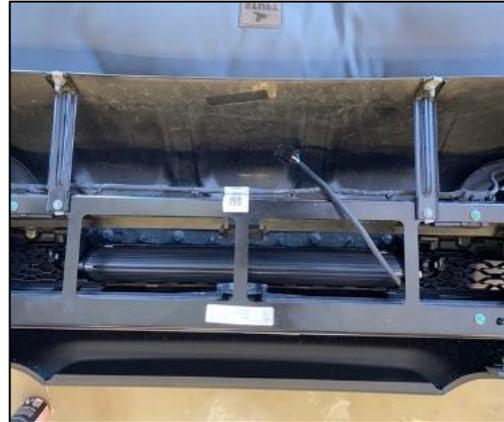
10. Using the existing hole location, Mount the bracket with the supplied 1/4-20 hardware.
