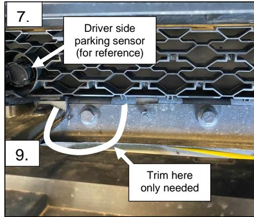
8. Unlock the clips on the top shroud allowing it to flex. (not completely removed) Pry open the should and rout the light bar through the opening.
